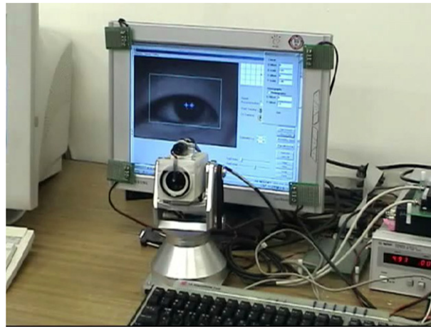
Fig. 22. Experimental setup: a monitor with four IR LEDs and two cameras mounted on a pan-tilt unit. A small wide-view camera is attached to the top of the high-zoom camera.
